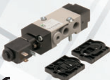
Convertible monostable solenoid valve IP65 KA0080ZB2.801 for 24VAC version KA0010ZB2.801 for 230VAC version
